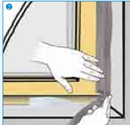
2 Make an 'ear' (fold, loop) at the corners, do this by pressing the window tape firmly into place up to approximately 2cm away from the corner, then slightly lift it and turn it 90° thereby creating a fold or loop that is then pressed back into the corner creating a 90° turning point for the installed tape.
