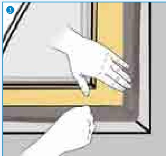
3 Continue to press the window tape onto the window frame. The 'ear' created will seal the corners perfectly. Repeat this procedure at every corner.
